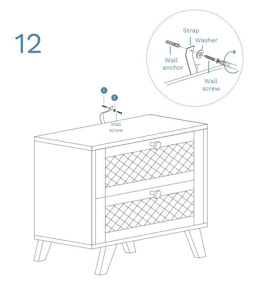
Once assembled lift furniture into place, do not drag. Use a drill to create a small hole lining up with the top of the safety strap (W). Fasten to wall using 1 x wall plug (X), 1 x washer (Z) and 1 x wall screw (not supplied).
