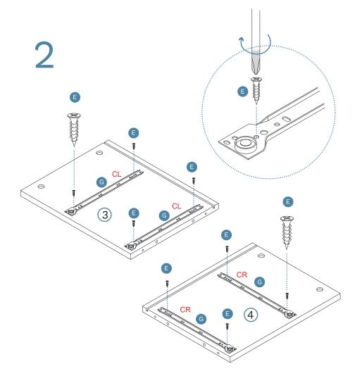
Attach 2 x left slide rails (G) to panel [3] and secure with 4 x small screws (E). Attach 2 x right slide rails (G) to panel [4] and secure with 4 x small screws (E). Tighten with a screwdriver.
