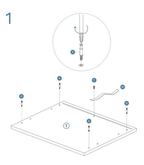
Attach 1 x wall strap (W) to panel [1] using 1 x screw (Y). Insert 4 x bolts (A) into panel [1]. Tighten with a screwdriver.
