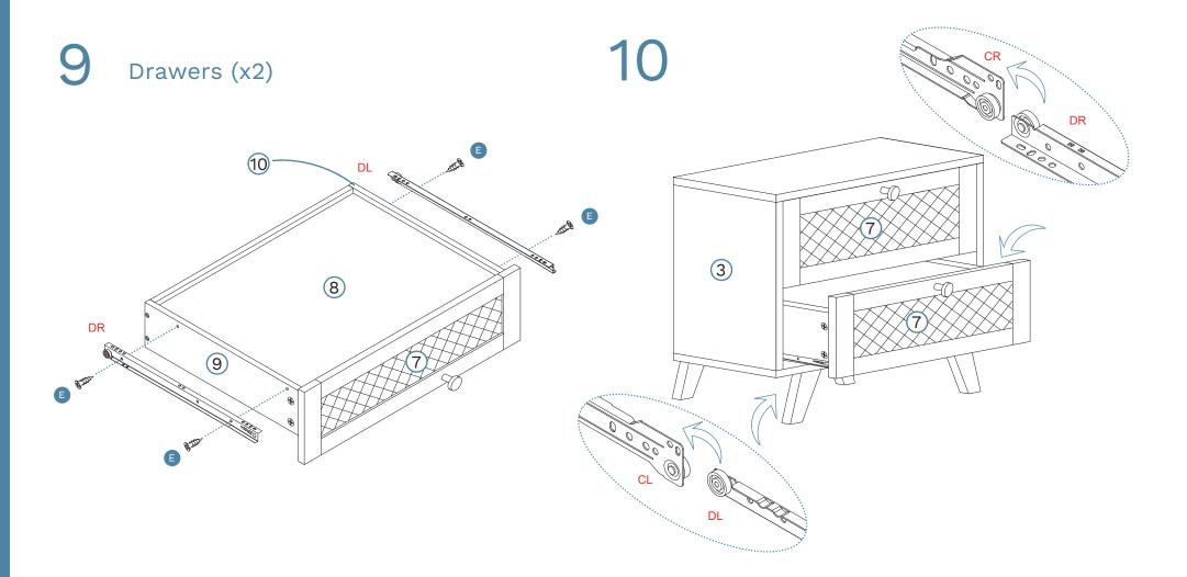
Attach 4 x slide rails (H) to panels [9] and [10], secure with 8 x small screws (E). Tighten with a screwdriver.
